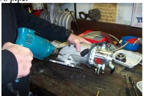
If retaining vacuum brakes drill here and tap to size.
