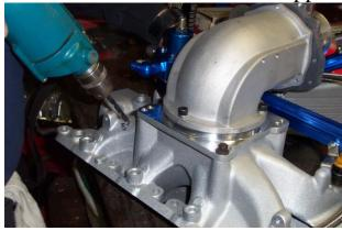
If using ACT sensor drill here and tap to 3/8 pipe.
