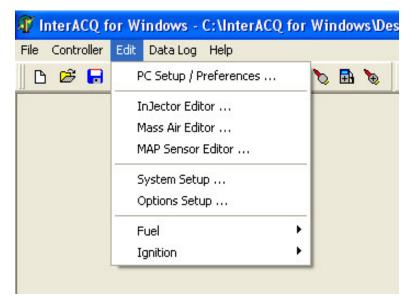
PC Setup / Preferences - This menu selection brings up a screen which allows you to set up parameters specific to your hardware or personal preferences. screen This contains four tabs labeled Forms & Menus, Monitor, COM Setup, and Export.
