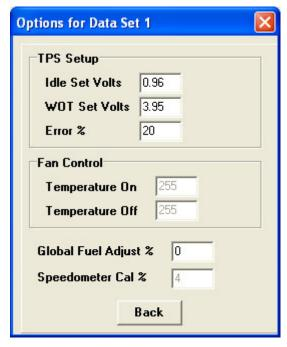
The **Misc Page 2 Setup** allows the user to make changes to the settings shown at the left. Not all applications support all of the adjustments.
