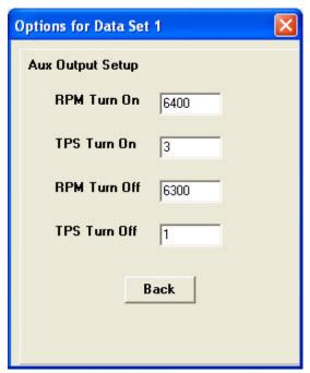
The Aux 1 and Aux 2 Output settings allow you to select the RPM and throttle positions at which the Aux 1 and Aux 2 switches on the PMS are turned on and off. To use these switches, you will need to follow the wiring instructions set forth in your PMS manual. The On settings may be greater than the Off settings or vice versa. For these settings to be effective, however, the TPS settings must be greater than zero.
