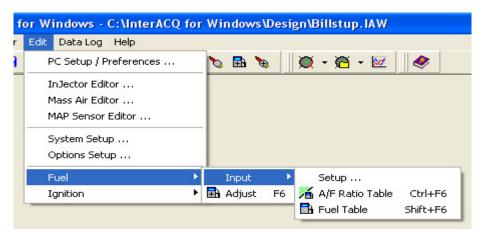
Setup - Selecting this submenu item will bring up screen allowing you to create a Stand Alone Fuel Input table to replace the default Fuel Input table in the PMS. (For information on using this screen see page 34.)
