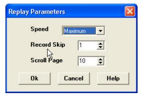
These parameters control the how the Review and Playback of the monitor data is displayed. Type CTRL-P to bring up the Replay Parameter dialog, or you can access via the **Parameters** options in the **Data Log** menu.
