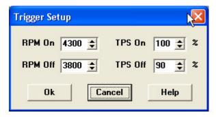
To setup the data monitoring triggers select Triggers from the Data Log menu, to type CTRL-T. This brings up the Triggers dialog box shown at right. Here you can enter the RPM and Throttle Positions where you want recording to begin and end. Enter the desired parameters and click "Ok." With the triggers set monitoring will begin automatically when the "On" conditions are
