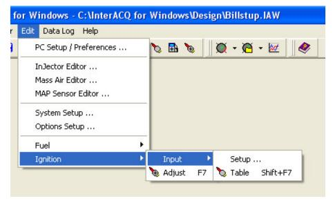
**Setup** - Selecting this submenu item will bring up screen allowing vou to create a Stand Alone Ignition table replace the default Ignition Input tabe in the PMS. (For information on using this screen see page 34.)
