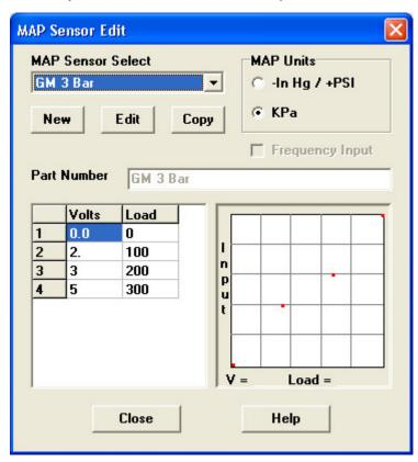
parameters (Voltage/Load Frequency/Load). Note: When the new data table is first presented it will have cells for Volt (or frequency) and Load at only one point. Additional points can be added by using the **Insert** keys to insert points, and the Delete keys to remove points. When you are finished click "Save." This will add the new MAP sensor to the list and return you to the MAP Sensor Edit screen with the new sensor as the active one.
