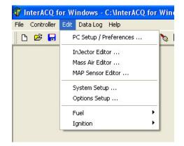
After making a connection to the PMS, select "System Setup, from the "Edit" menu. This dialog box will show the engine's defaults from the PMS. Typically, you will only need to access or modify these settings when you first setup the program or when you change your injectors or mass air meter. You may also use this screen to change the default Data Set, Password or display Units for the monitoring
