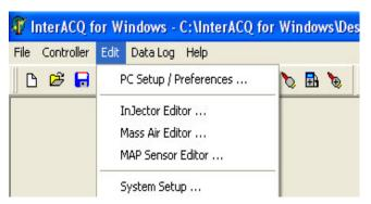
Go to the "Edit" menu and select "PC Setup/Preferences." Set-up is normally necessary only when using the program for the first time, although you may decide to change the Monitor tab options and the new Auto Connect option under COM Setup tab occasionally. The PC Setup/Preferences dialog box will be displayed.
