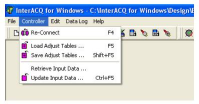
Connect or Re-Connect - Use this menu selection, the F4 key or the "Connect" button on the tool bar to initiate (or re-initiate) the process of connecting InterACQ to the PMS Controller.
