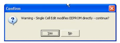
**CAUTION -** Unlike editing the Anchor Points, where no change is made in the EEPROM until the change is saved, changes made in the Single Edit mode **alter EEPROM immediately.** This must occur to maintain the "line" or "curve" between the Anchor points, as discussed in Adjust Table Edit. When you alter an intermediate data point you are in effect creating your own "curve" between the anchor points. Keep this in mind and use caution when making changes in the Single Edit mode.
