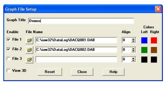
The Setup button will display the Graph Setup dialog, used to select and load the monitor data files. This dialog is used to load the files for graphical display. Up to three files can be selected simultaneously.
