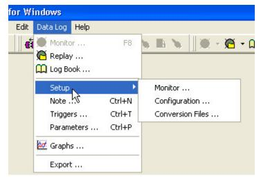
Monitor –The Monitor Setup menu selection will allow you to customize the look and feel of the Monitors. The program includes a Default graphical Monitor and a Text Monitor. Either of these Monitor forms can be edited or you can create a fresh Monitor design. For more information on how to use this function, see page 45.
