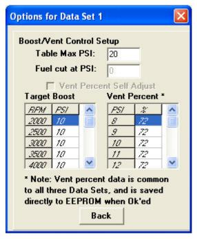
boost exceeds the setting. The **Target Boost** and **Vent Percent** settings are used together to give the PMS control of the turbo wastegate to establish a targeted level of boost. The **Vent Percent** settings are used in all three Data Sets to view or set the wastegate values, if one chooses to do so, automatic Vent Self Adjust can be turned off, and the Vent Percents set manually.
