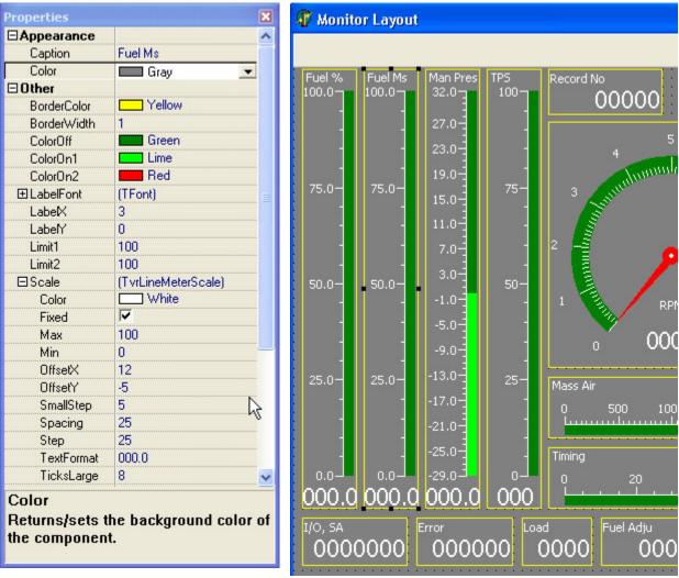
You can also move and re-size all the items in the Layout Form. Click on an item, but while holding the left mouse button down, move the mouse. The item will follow the mouse. To re-size, click on one of the anchors (little black squares) and again while holding the left mouse button down, move the mouse.
