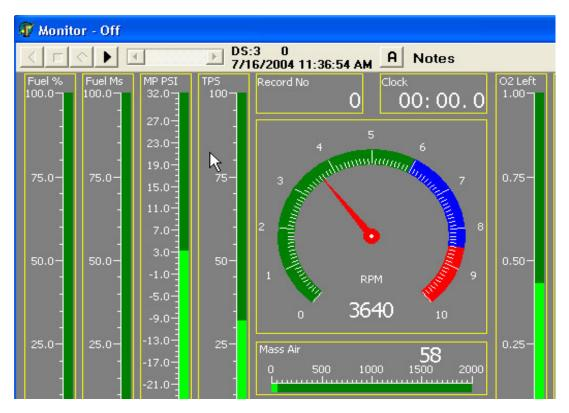
Shown above is a portion of a typical Monitor Screen or Form. All Monitor and Playback screens have the same controls across the top used to control the Monitor process, playback navigation, and to display useful information. At the upper left, there's a set of buttons (some are grayed out) similar to those on a VCR, to **Start / Play, Stop, Pause, and Rewind** the monitoring sequence. Next to the buttons is a scroll bar for navigating
