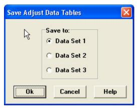
Adjust Data Tables" dialog box. This dialog box allows you to select the PMS Data Set (1, 2, or 3) that you want to save to, just as with the PMS hand held data terminal. To save to a Data Set, select the Data Set number. You may also load a different Data Set as with the Hand Held Terminal. From the "Controller" menu, select "Load Adjust Tables". The dialog box shown at right will appear where you can choose the Data Set (1,2, or 3).
