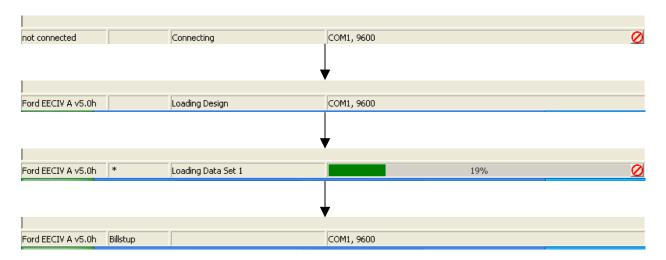
If there is a Design File previously saved on the PC, InterACQ for Windows will load it from the hard drive. However, if the Design File on the PC is newer or older than the data stored in the PMS's memory a "Warning" dialog box will appear and notify you that InterACQ will use the input data stored in the PMS's memory instead. This will not happen if the Design File and the data in the PMS have the same time/date stamp.
