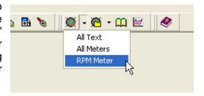
The Monitor screen displays graphically or as text RPM, Timing, Fuel, Throttle Position, Oxygen Sensor Voltage(s), Mass Air Flow or Vacuum Manifold Pressure, Water Temperature, and Air Temperature, plus other data. If the Stand Alone feature has been enabled and set up, then Load, Volumetric Efficiency, and Estimated Horsepower may also be displayed. There are several ways to use the Monitor feature.
