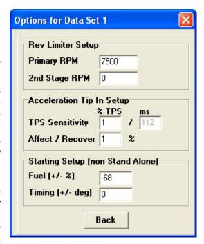
startup for the amount of time appropriate for stock injectors. If larger than stock injectors are used, however, a shorter pulse width will be appropriate to deliver the right amount of fuel. Experiment with this setting when the engine is cold and when it is warm to see what works best for your combination.
