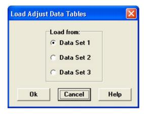
If you want to work on a different Data set, go to the "Controller" menu and select "Load Adjust Tables." This will bring up the "Load Adjust Data Tables" dialog box. This dialog box allows you to select the PMS Data Set (1, 2, or 3) that you want to load. Once you click OK, the program will then re-read the Adjust Table data from the PMS (similar to what happens when you Connect).
