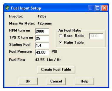
Select the RPM and Throttle Position Turn On points (that is, where you wish the Stand Alone feature to take over), the Starting Fuel (in milliseconds) and Fuel Pressure, and whether or not you want to use a Base Ratio or the Ratio Table ("Ratio Table" is the default and is suggested for ease of use). When this is done click "Create Fuel Table" and InterACQ will create the Fuel Input Table and Air Fuel Ratio Table.
