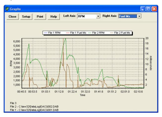
The Left/Right Axis combo boxes lets you select what parameter to graph using the left/right axis. Selections include RPM, Timing, Fuel Pulse Width, Fuel Percentage, Load, and all the analog inputs (TPS, O2, etc)
