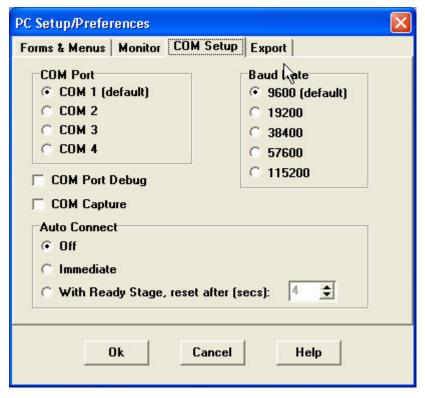
Select the **COM Setup** tab and then select the COM Port and Baud Rate (data transfer rate) desired. The default settings of COM 1 and 9600 Baud recommended unless there is a specific need to change it. The new Auto Connect explained is more fullv The choices here below. are Off, Immediate and With Ready Stage. Select **Off** for now. The **Ready** again after selection box is also more fully explained below and only impacts the With Ready Stage option.
